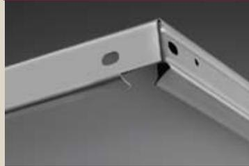
Shelf corners are fully lapped and welded for extra strength. Combined with sides that incorporate triple-bend construction, shelves can support up to 1,000 pounds.
